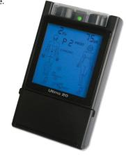
**MODE BURST A** — One train any 3 seconds, 1s on, 2s off. Both Pulse Rate and Pulse Width are freely adjustable. Default values are PR=30Hz and PW=250\_s. The stimulation level must be set to produce a gentle muscular contraction.
